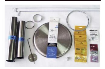
Stove body: 36 of 12 inches stainless steel or titanium foil makes a 12-inch long stove and will work for up to a 10.25-inch diameter stove. If you want a longer stove you can order 16- or 22-inch foil by the same length.
