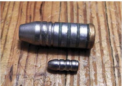
flame heat source is in use. Maybe most importantly, keep all water sources away from your molten lead. Water vaporizes instantly when it contacts the 600-degree lead, and the resulting expulsion of steam can send melted lead droplets in every direction.
