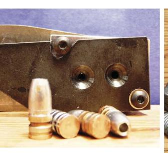
antimony are available from many on-line sources for customizing the hardness of your bullets. The general rule is, the faster the bullet, the harder it needs to be to prevent it from shedding lead down the gun barrel. Most wheel weights measure around 12 BHN, which is perfect for most standard handgun loads.
