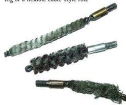
(above) Clearly the effectiveness of these brushes has long since passed. (right) Cleaning rod tips come in two basic types: slotted tips and jags. They are most often made of aluminum, plastic or brass. Either style does a great job, so which type you choose to use is simply a matter of personal preference.
