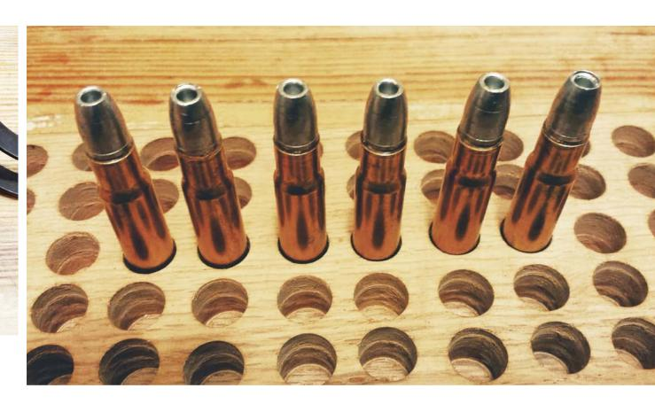
tant to keep your molds from becoming too hot during the process. A sure sign of excessive heat in the mold is the formation of a frosty grey finish on the cast bullets. If you notice a discoloration of your bullets, simply set the mold aside for a few minutes to cool. This problem can be overcome through the use of two molds, alternating with each pour so that the molds have time to cool just a bit between fills.
