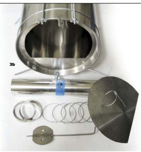
washer and wing nut to each of the body support rods. Standard 1" washers can be used if you put a 135-degree bend in them so they grip the end plates. A better option is using obtuse corner cabinet brackets—they are lighter and the bend is perfect but they can be harder to find. Use pliers to mess up the threads behind each wing nut—this will eliminate the chance of losing any small parts.
